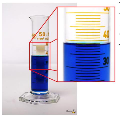
The measured value is read off at the level of the phase boundary (below the meniscus if there is one).
