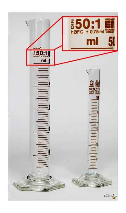
Typically, all volumetric instruments are provided with details regarding accuracy and application.
